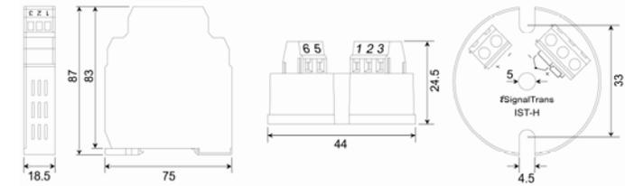
Figure 1. Dimension in mm
