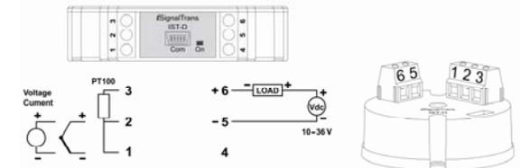
Figure 2. Terminal connections
